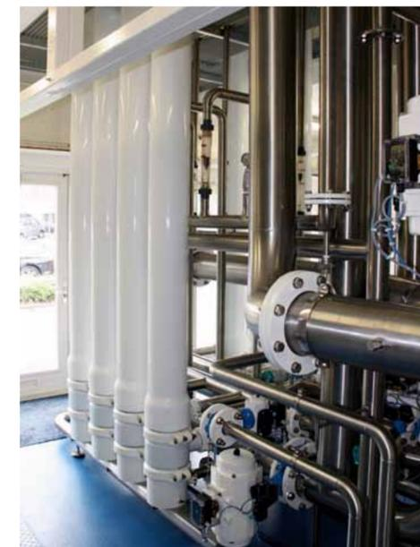
hospital wastewater. The Paques downstream membranes were compared to an upstream system with air injection from below. It appeared that the downstream membranes, with air intake from above, showed permeability twice as high for only a third of the energy consumption. Finally, the side-stream membrane installations as the BIOPAQ® MBR are inherently more hygienic than submerged membranes and the maintenance is easier and costs, especially with the new downstream membranes, much less time.
